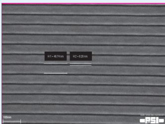
12 nm trenches, 50 nm pitch, imprinted in mr-I 7000R (Courtesy of Eulitha AG and Paul Scherrer Institute)
